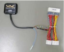
Coupler-on Harness Length: 150 [mm] Main Unit Harness Length: 250 [mm] Main Unit Size: 60 × 63 × 15 [mm]
