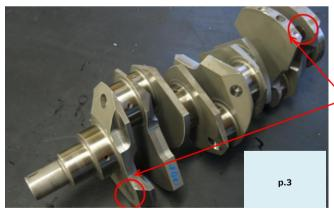
By using the heavy alloy Amviroy® for counter weight, it can restrain the vibration without increasing the volume of counter weight itself.
