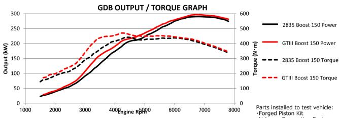
297kW (400ps) /6700rpm 470N·m (48kgf·m) /4300rpm generated when boost set to 150kPa with EVC.
