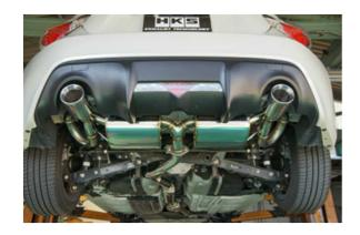
SUPER MANIFOLD with CATALYZER R-SPEC
