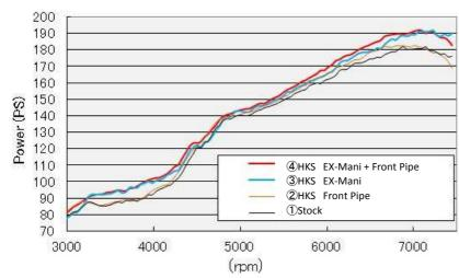
As you can see on the left graph, the exhaust manifold is the main part for the higher output.
